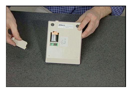
Remove the battery rate chip compartment cover from the bottom of the scale.
